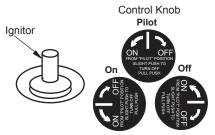
Figure 21 - Ignitor and Control Knob
